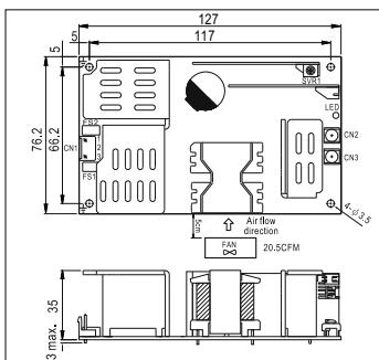
AC input voltage range ..... 90~264VAC; 127~370VDC
