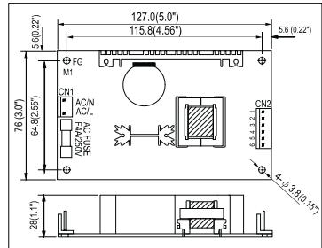
AC input voltage range ... 90~264VAC; 127~370VDC
