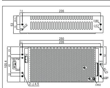
AC input voltage range .....90~264VAC; 127~370VDC
