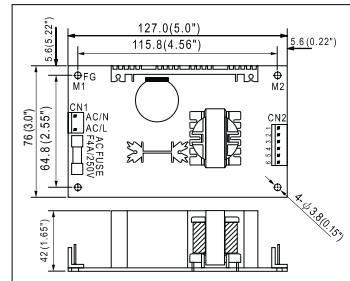
AC input voltage range ..... 90~264VAC; 127~370VDC
